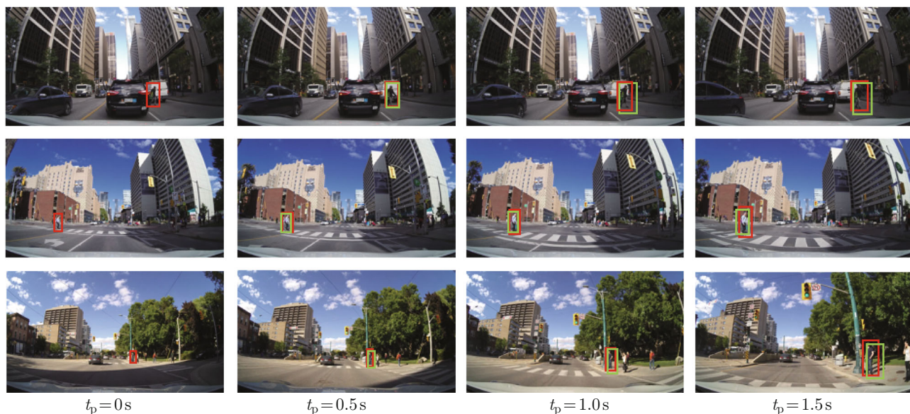
Fig. 4 Visualization examples of pedestrian trajectory predictions (red for ground truth and green for prediction)
